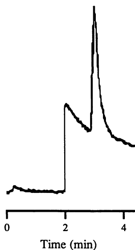
Figure 12. Analysis of Bromacil. Bromine II: 478.55 nm, Two section tube: "inlet tube": 1 mm i.d., "plasma tube": 3 mm i.d., Absorbed power: 230 W. Gas flow rate: 50 mL/min. Chromatographic conditions: Packed column: 1.8 m, 2 mm i.d., SE-30 5% on Chromosorb W-HP 80/100 mesh. Isothermal separation. Temperature: Oven: 220 °C, Injector: 280 °C and Interface: 350 °C.
