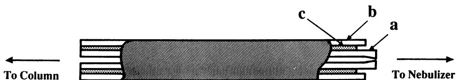
Figure 2. Schematic diagram of restrictor. Components: a=Pyrex glass capillary (35 mm x 50 \mu\text{m} i.d., 0.5 mm o.d.) with an opening of ca. 5 \mu\text{m} , b=stainless steel tube (34.5 mm x 0.8 mm i.d., 1/16 in.o.d.), c=epoxy resin.
