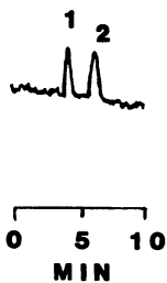
Figure 6. HPLC-DCP chromatogram of feed premix sample containing nominally 100ppm Se each as selenite and selenate species, HPLC-DCP conditions as in Figure 4. Peak identities: 1 = selenite; 2 = selenate.
