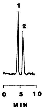
Figure 4. HPLC-DCP chromatogram for the separation-detection of selenite and selenate species under paired-ion, RP conditions: C-18 column (10 \mu m, 15cm x 3.9mm i.d.); mobile phase of 2.5mM TBAHS, 0.01M each dipotassium hydrogen phosphate and potassium dihydrogen phosphate, pH = 6.55; flow rate 0.5ml/min; DCP detection at 196.026nm; injections of 50ul of 20 ppm each Se species as standards. Peak identities: 1 = selenite; 2 = selenate.
